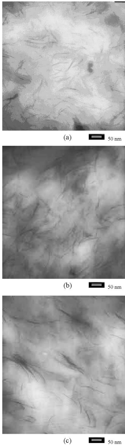
Fig. 3. TEM micrographs of the composites: (a) PA 6/30B; (b) PA 6/30B/POEMA; (c) PA 6/30B/POEMA*.
